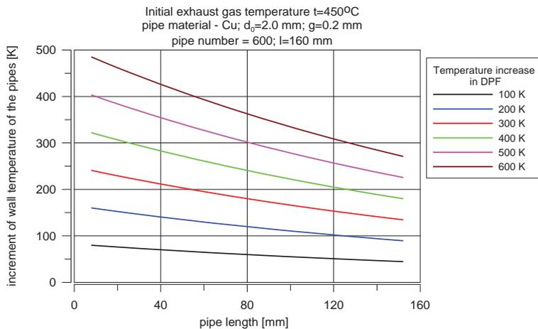
Fig. 7. Increment of the wall temperature at different temperature increment in DPF for copper pipes at initial gas temperature  $450^{\circ}\text{C}$  without radiation
