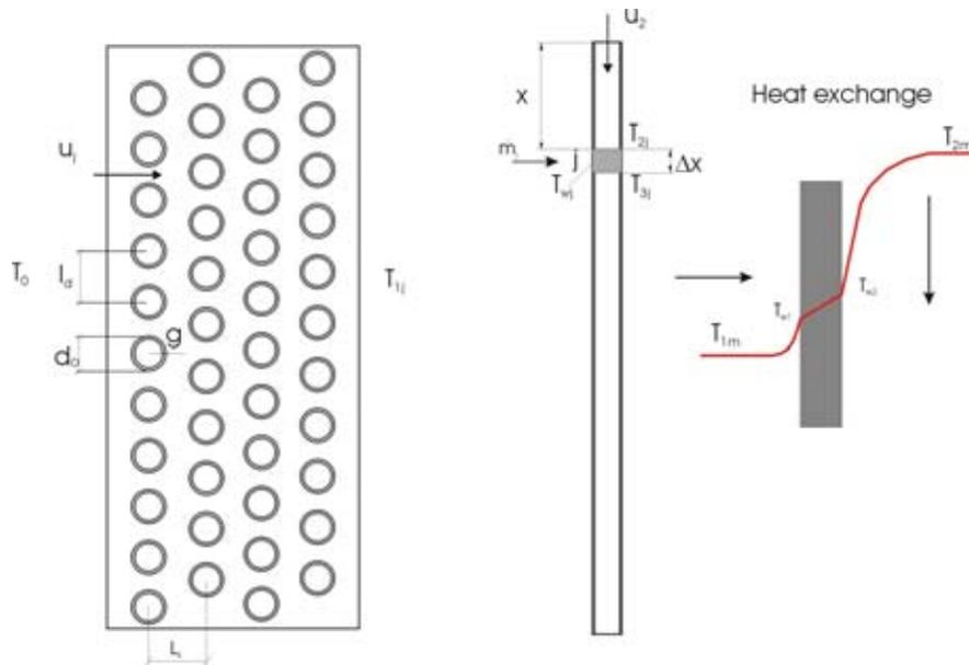
Fig. 3. Heat exchange on the discretization model
