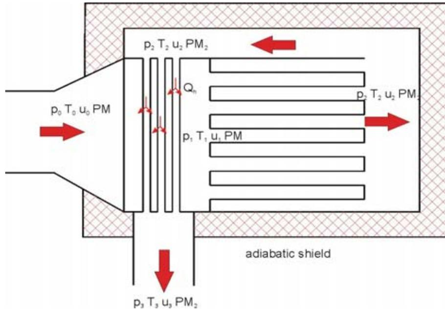
Fig. 2. Diagram of the DPF regeneration model
